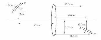
34.116: a) Using the diagram and law of sines  $\frac{\sin \theta}{(R-f)} = \frac{\sin \alpha}{g} \text{ but } \sin \theta = \frac{h}{R} = \sin \alpha \text{ (Reflection Rule)}.$ So g = (R-f). Bisecting the triangle:  $\cos \theta = \frac{R/2}{(R-f)} \Rightarrow R\cos \theta - f\cos \theta = \frac{R}{2}$
